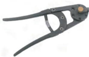
ATI501R This rivet cutter is designed to quickly and easily shear aluminum rivets. It is adjustable for 1/4" to 3/4" long rivets in 1/16" increments, for rivet sizes 3/32", 1/8", 5/32", 3/16", 7/32", and 1/4".
