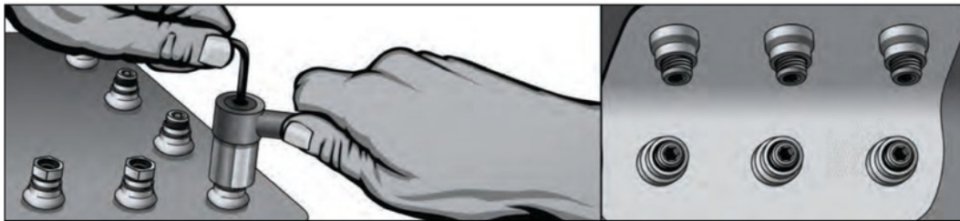
Installing the Hi-Lok® fastener with the "Roller Clutch" wrench.
